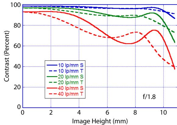
Figure 4: MTF at 10, 20, and 40 lp/mm for f/1.8
