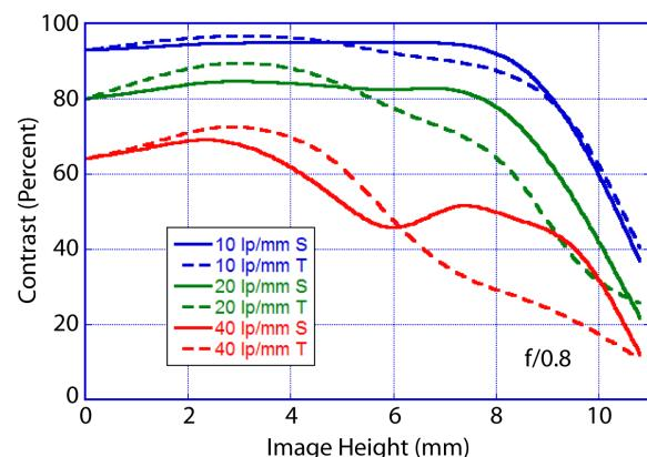
Figure 2: MTF at 10, 20, and 40 lp/mm for f/0.80
